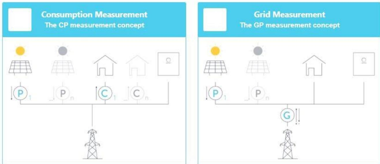
**Consumption Measurement** will calculate power flow both in export and import from the grid metering point. This calculation is based on the measurement of the solar PV production as well as the load consumption at the closest point to the loads. This calculation will also factor the input and output of the sonnen eco 8 system allowing for all conversions from AC to DC and reverse, plus system self-consumption.
