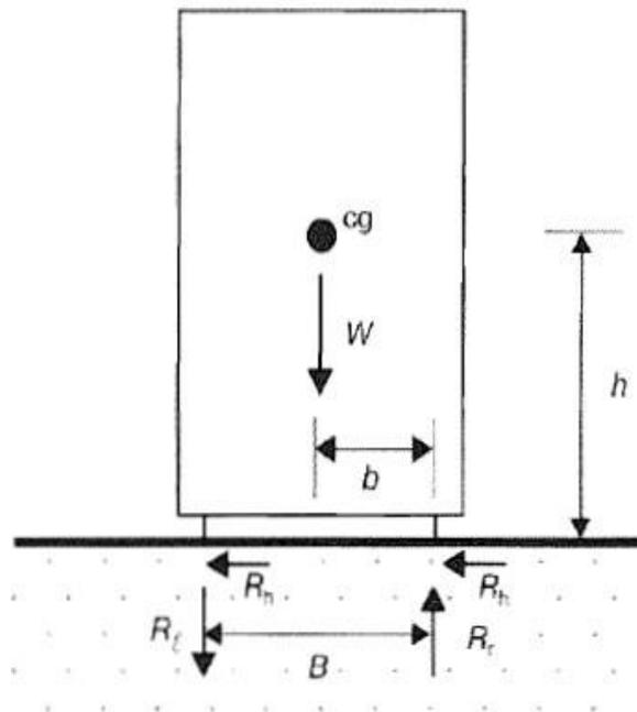
The overall requirement is to determine the number and size of hold-down anchors / fixings utilised and/or in addition to the standard fixings detailed by sonnen.
